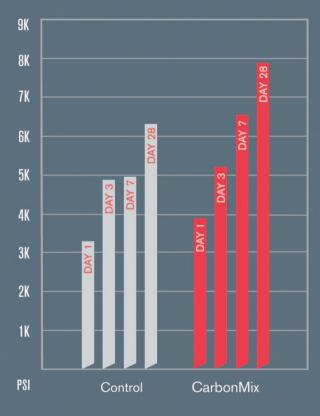
CONCRETE DATA 4" X 8" CYLINDER COMPRESSIVE STRENGTH
